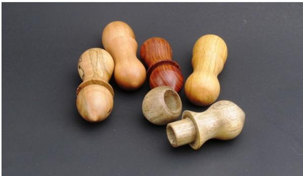
**Variations:** Needle case blank 5.25" with finished needle case 3." 1 3/4 was needed for waste wood for tenons, parting off and for the overlap of the cap on the body of the needle case. Make it about 3 3/4" long using 1/2" and 3/8" drill sizes for a traditional needle case. For toothpicks (2 1/2"), 19/64" BS 1/2" drill bits with a blank about 7/8" x 3 1/2."
